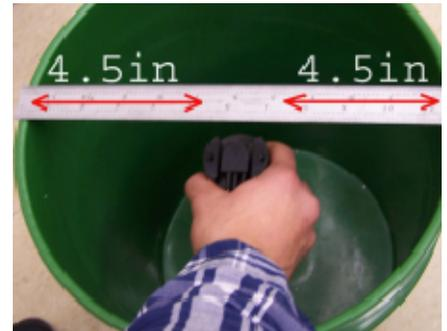
*Minimum container size for low level system verification. Not intended for high drive level operation. Do not operate in air.*
